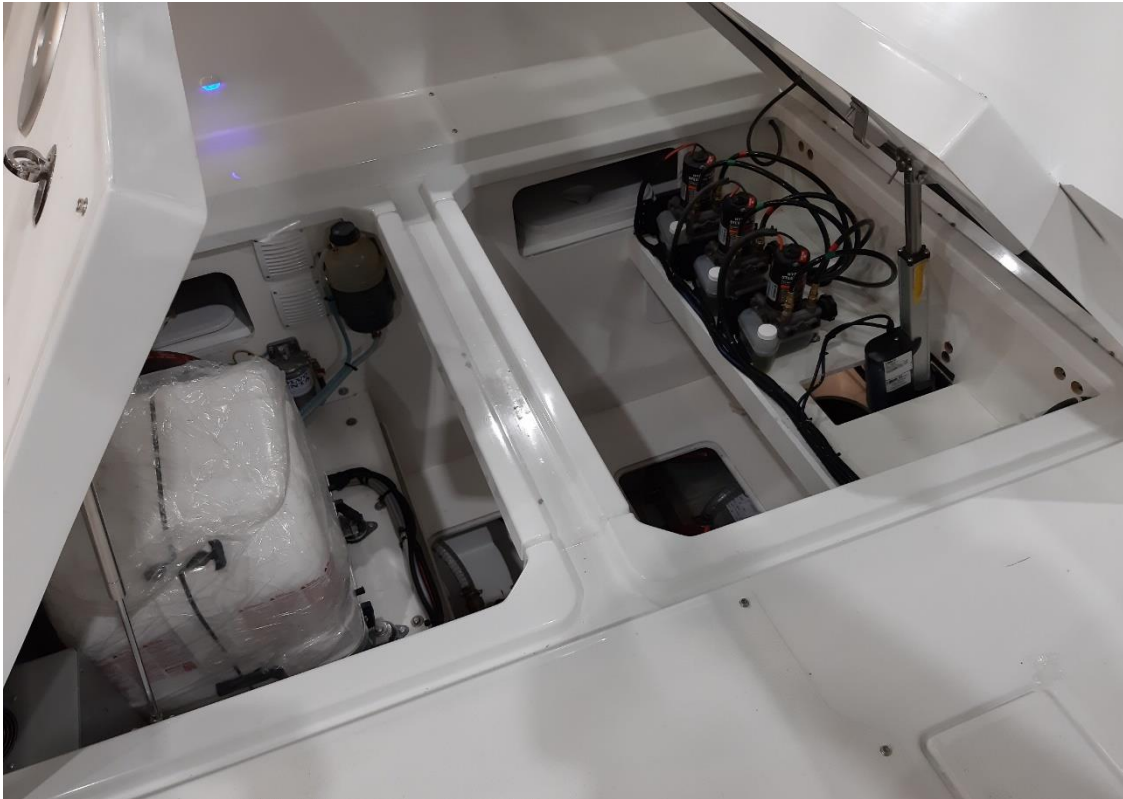
Option : Fischer Panda 6,4 KVA generator with dedicated tank (30L / 8 US Gal) + deck fill
