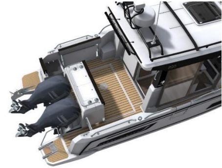
Sliding aft bench : enables to lift up the engines and keep the seats
