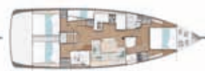
Version E Forward owner's cabin, 2 aft cabins, 1 port side lateral cabin / 2 heads
